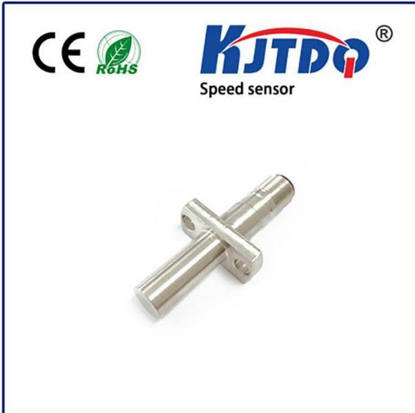
The KJT D12A series Differential Hall-Effect Speed sensors are suitable, in conjunction with a ferrous pole wheel, for generating square wave signals proportional to rotary speeds. It exhibits a static function, whereby pulse generation down to 5 Hz is guaranteed.
