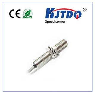
KJT's zero speed hall effect sensors for measurement of hub speed and shaft revolutions, etc, with an internal magnet to switch in the presence of ferrous targets such as gear teeth and blade tips down to absolute zero speed. It detects fluctuations in the magnetic field and can also be configured so the output signal signifies either the presence or absence of a ferromagnetic target (i. e. A gear tooth, shaft feature, etc).
